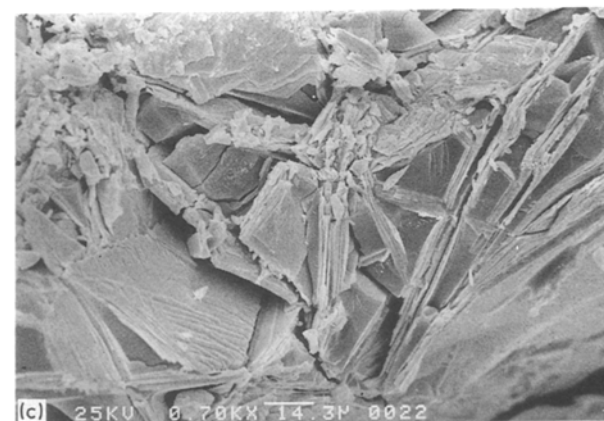
Figure 6 Scanning electron fractograph of sintered sample depicting densification steps (a) sintering at 1250 °C for 5 min, (b) sintering at 1350 °C for 5 min and (c) sintering at 1550 °C for 5 min.
