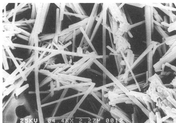
Figure 5 Scanning electron fractograph of sample sintered at 1100^\circ\text{C} for 24 h showing a crystalline structure with no apparent densification.
